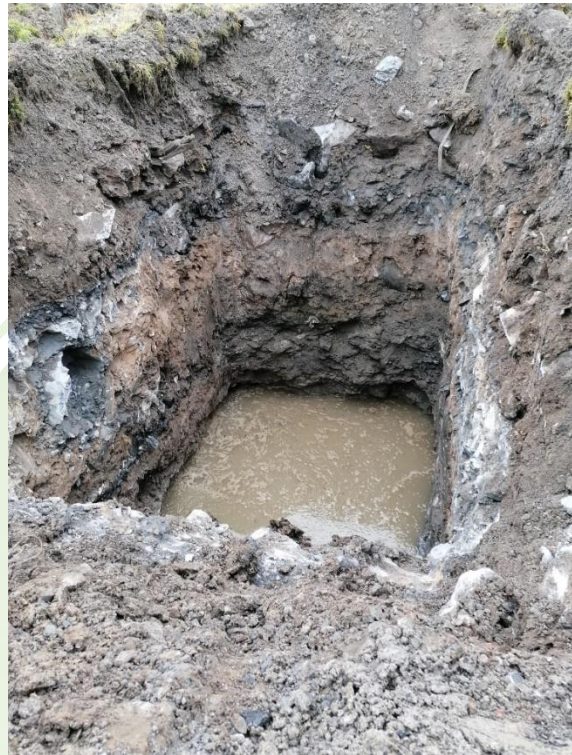
Figure 6: Illustrates trial hole 1 & shows the different horizons within the trial hole.
