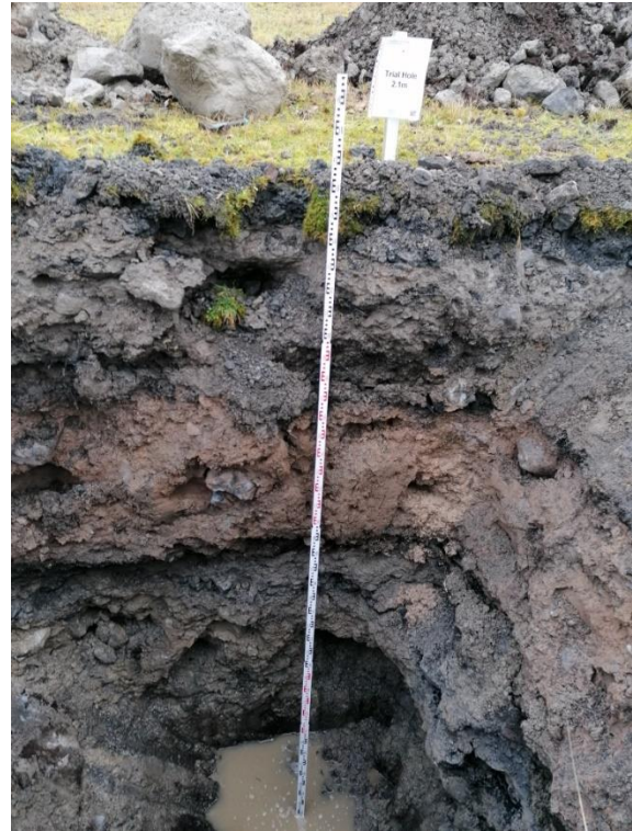
Figure 12: Illustrates trial hole 1 & shows the different horizons within the trial hole.
