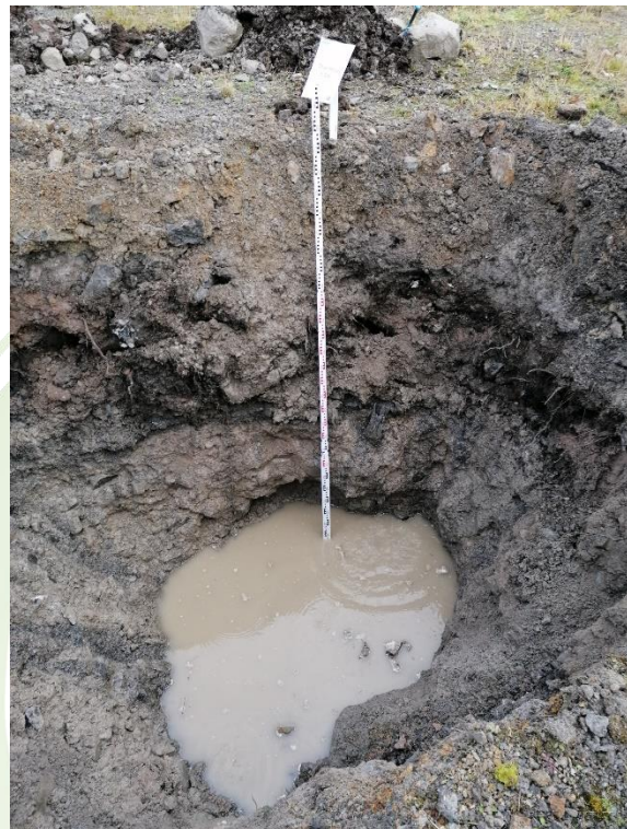
Figure 30: Illustrates trial hole 5 & shows the different horizons within the trial hole.
